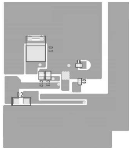
Back Side: GND Side (double sided board)
